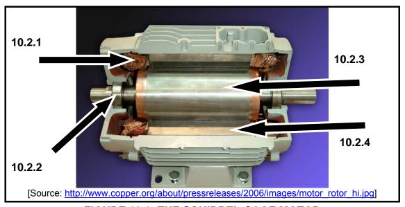
FIGURE 10.1: THE SQUIRREL-CAGE MOTOR
