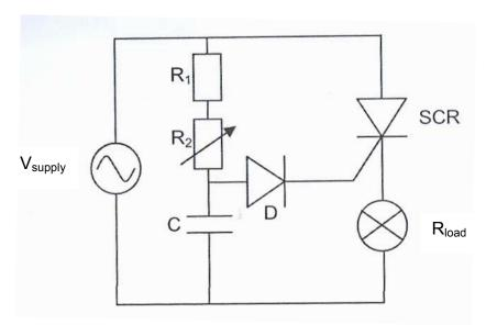
FIGURE 6.1: LAMP DIMMING CIRCUIT
