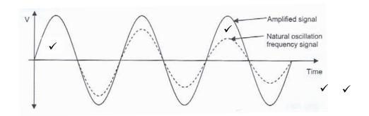
The electrical signal that the oscillator produces is called the natural oscillation frequency. ✓ Natural oscillation diminishes in amplitude and disappears due to a lack of positive feedback ✓ We decided that three marks should be for the diagram and three marks for the explanations.
