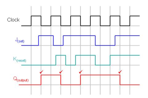
All changes to output Q must be in line with the enabling clock pulse no matter when input changes. Note the order of change. First either J or K is set or reset, then the clock pulse enables the output to change accordingly.
