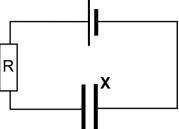
Capacitor **X** is now replaced with a similar capacitor, **Y**, with the same dimensions but with paper between its plates. When fully charged, the charge stored on the plates of capacitor **Y** is ...
