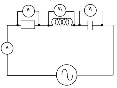
FIGURE 5.1 – RLC SERIES CIRCUIT
