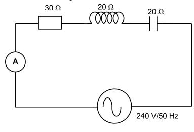
FIGURE 5.3 – RLC SERIES CIRCUIT
