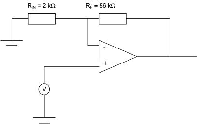
FIGURE 7.2 – NON-INVERTING AMPLIFIER CIRCUIT
