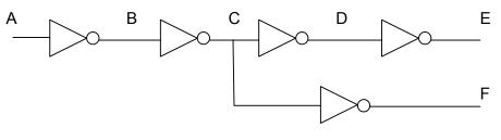
**FIGURE 9.1 – CASCADE INVERTERS**
