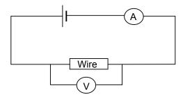
The potential difference across each wire is increased in equal increments, and the resulting current through these wires is measured. Using the measurements, the learners obtained the following sketch graphs for each of the wires.
